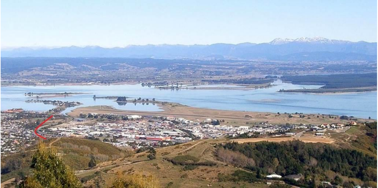
Fig. 1. Tahunanui area. The red line (left) is the 7,000 year sea cliff extending from the Annesbrook roundabouts to the base of the spit forming Monaco. North of the sea cliff the low-lying land is dominantly marine sands with gravel adjacent to the toe of the Port Hills.
