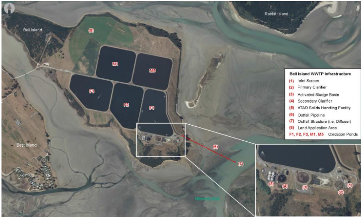
Figure 8-2: Main components of the WWTP (from Bell Island WWTP Application and AEE 2017)
